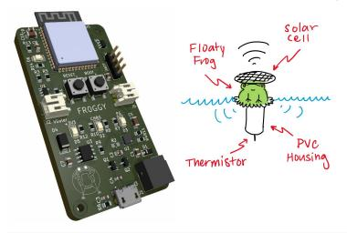
**Objective:** Develop an IoT floaty pool thermometer to transmit pool temperature over Wifi.
